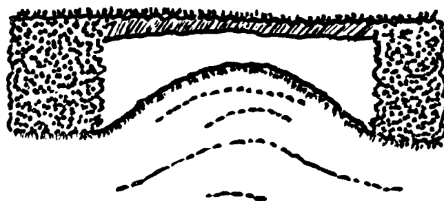
Fig. 23. Character of the filling of the gasified space due to sagging of the roof rocks.
