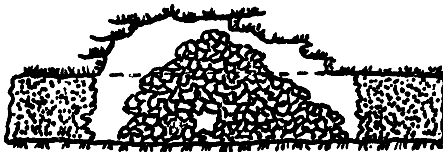
Fig. 24. Character of the filling of the gasified space by the collapse of the roof rocks.
